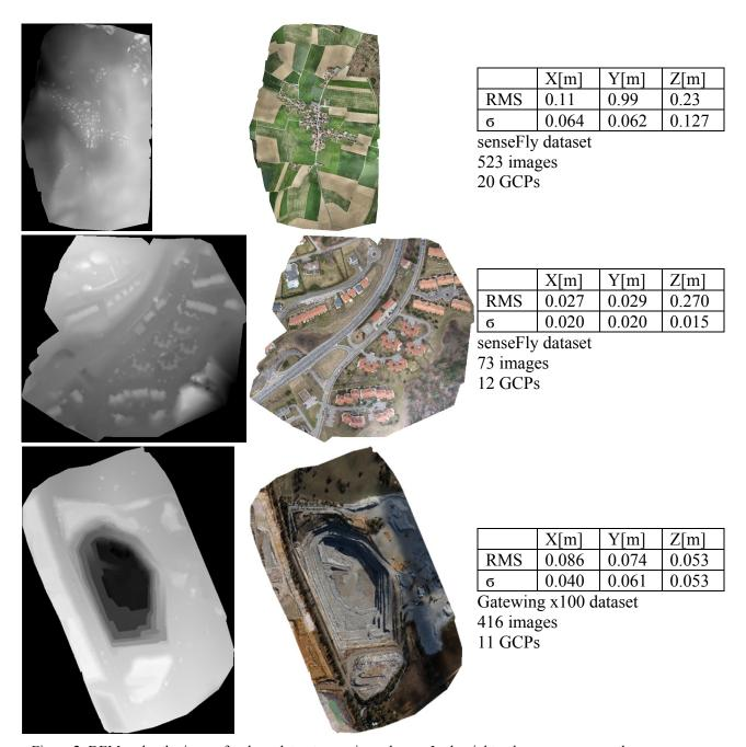
Figure 2: DEM and ortho image for three datasets, one in each row. In the right column one can see the mean errors and their variance in each dimension for all GCPs.
