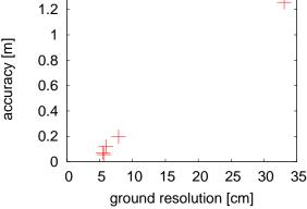
Figure 1: Dependency of the accuracy from the ground resolution (Ground sampling distance) of the original images for various datasets with using GCPs (left) and without using those (right).
