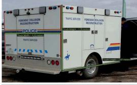
Images acquired by the UAVs were processed and the threedimensional scene was reconstructed by Pix4Dmapper. As seen in the lower graphs, we measured the width, length, and height of the RCMP truck directly in the software, and the results exactly match the real RCMP truck dimensions.
