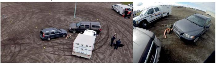
The project took place in Regina, Canada. A staged car accident scene was set up to reproduce a crash of two vehicles with a person fallen out of one of the vehicles. The RCMP took photographs and measurements before anything was moved. The yellow plastic evidence markers indicated where each piece of evidence was found.
