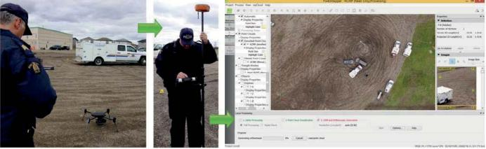
The whole procedure can be completed right after the accident occurred, including the on-site flight and an additional ten minutes of optional but recommended measurements for quality assessment. For this project, the total processing time of Pix4Dmapper was approximately two hours. After processing, the whole scene was reconstructed and the terrain model, point clouds, and orthomosaic were exported. Annotation and measurement were then directly performed in the software.
