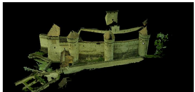
Figure 11. Results of the bundle adjustment. Automatic tie points, GCPs, and camera centres shown in rayCloud Editor for the Sony Alpha7R with 16mm fisheye lens
