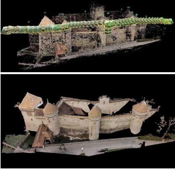
Figure 22. Results of the bundle adjustment. Automatic tie points, GCPs, and camera centres shown in rayCloud Editor (top) and the resulting dense point cloud (bottom)
