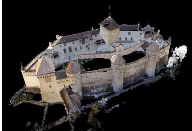
Figure 10. Results of the bundle adjustment. Automatic tie points, GCPs, and camera centres shown in rayCloud Editor (top) and the dense model at the bottom for the Sony Nex 7
