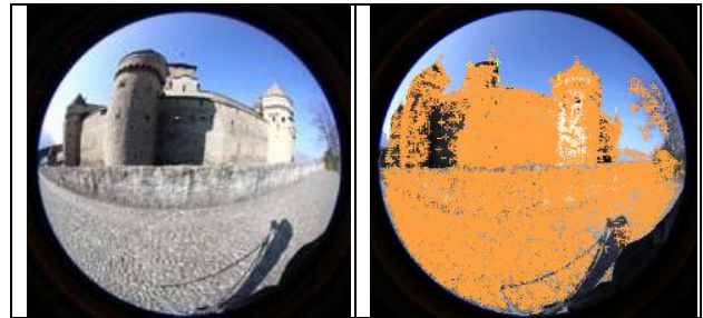
Figure 15. Canon 6D with Sigma fisheye 8mm example. On the right one can see the automatically extracted and geometrically verified key-points after bundle adjustment. The distribution up to the border of the image indicates the correctness of our fisheye camera model
