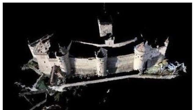
Figure 17. Results of the bundle adjustment. Automatic tie points, GCPs, and camera centres shown in rayCloud Editor
