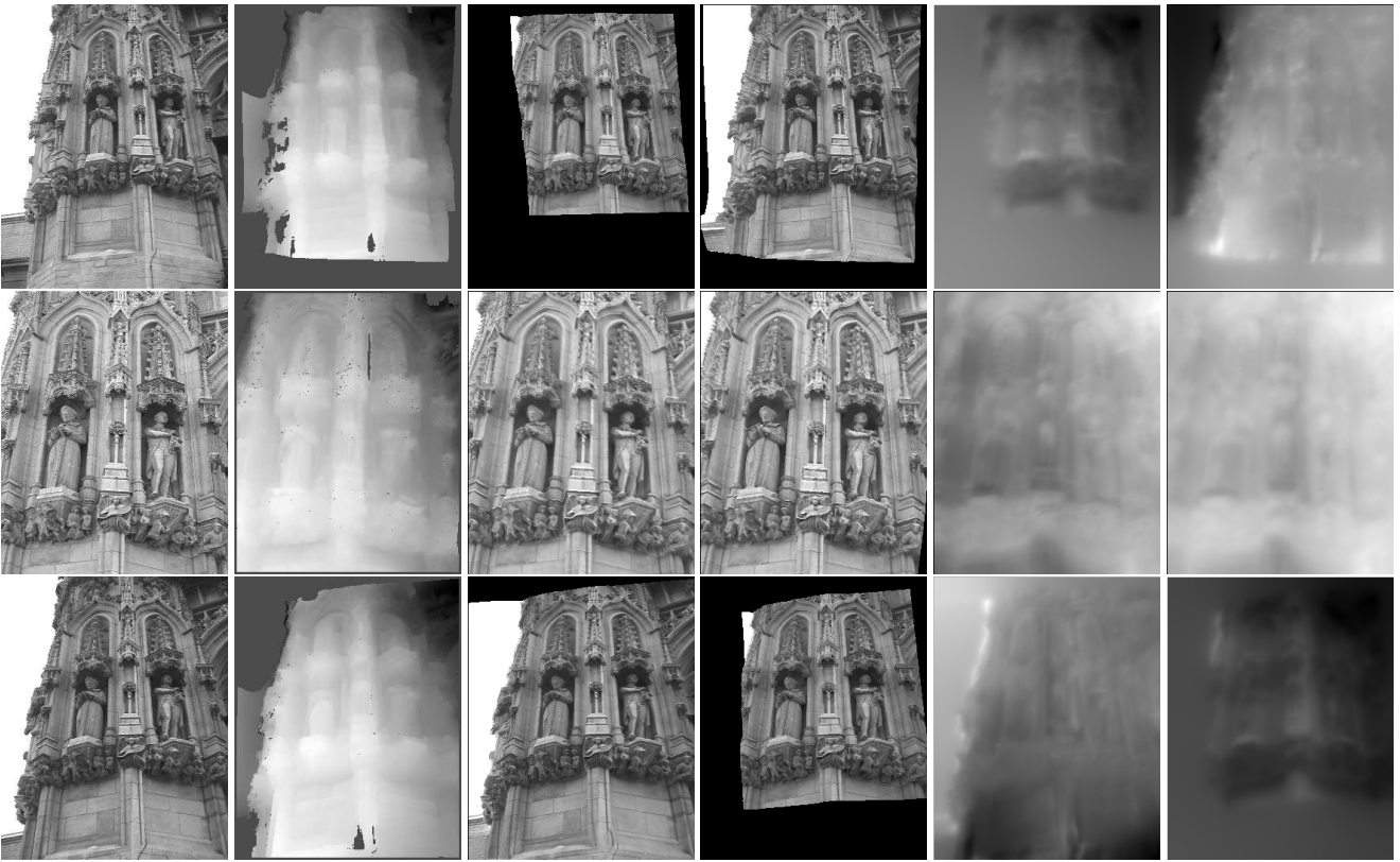
Figure 6. Intensity scaling experiment: from left to right (a)-(f) In each row: original image(a); inverse depth map(b); (c,d) the two images(a) from the other rows warped to the image(a) in the row taking into account their depth maps and the intensity scalings \kappa_{ij} ; the intensity scalings \kappa_{ij} (e,f) that accounts for the light change from the two images(a) of the other rows to the image(a) in the row ( \kappa_{ij} maps).
