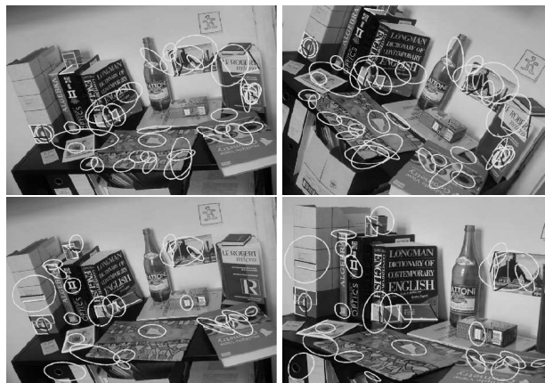
Figure 1. 3 wide-baseline views of the ‘bookshelf’ scene. Top: images 1 and 2 with matching invariant regions; bottom: the same for images 1 and 3.
