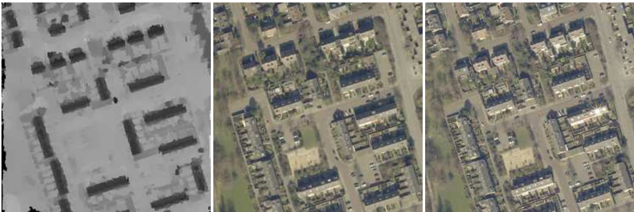
Figure 5: Expected value of depth (left) and the estimated orthoimage y^* (middle). One of the input images is shown right. Note that the specular reflection of the sun in the input image. This disappears in the estimated orthoimage.
