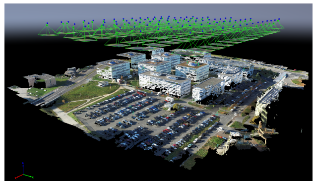
Figure 1: Screenshot of the Pix4Dmapper reconstruction of our test site for a dataset recorded with a DJI Inspire 1.
