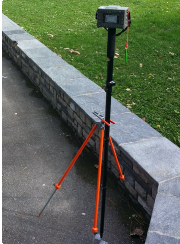
Figure 9: The Javad Triumph-LS receiver was used to measure the positions of checkpoints.
