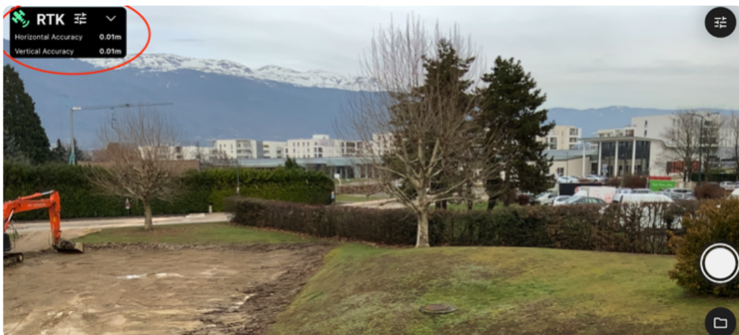
Figure 7: The capture screen of Pix4Dcatch displays the real-time accuracy once connected to the RTK rover.
