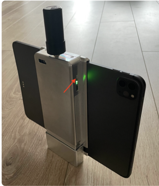
Figure 5: Power button located on the side of the RTK device.
