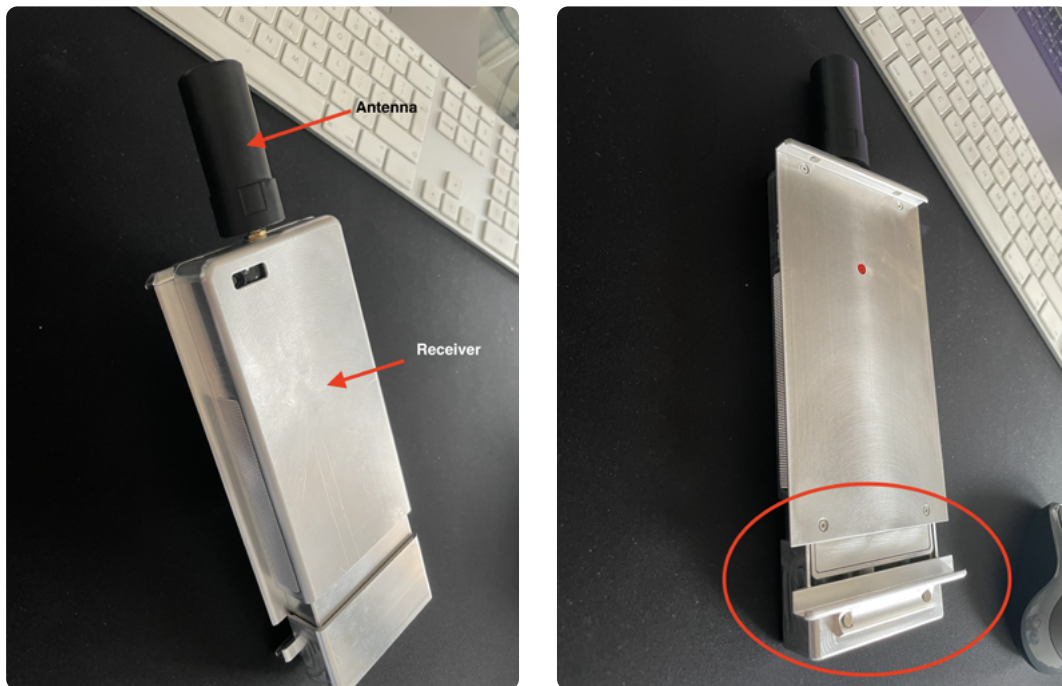
Figure 2: The viDoc® RTK rover for iPad - left: The two main components (antenna, receiver) are indicated with the red arrows. Right: Adaptable RTK rover for iPads.
