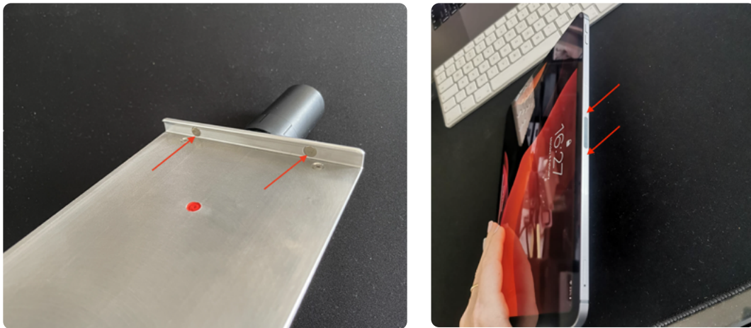
Figure 4: Left: The small magnets on the viDoc® RTK rover (indicated by the red arrows). Right: Position of the iPad's magnets.
