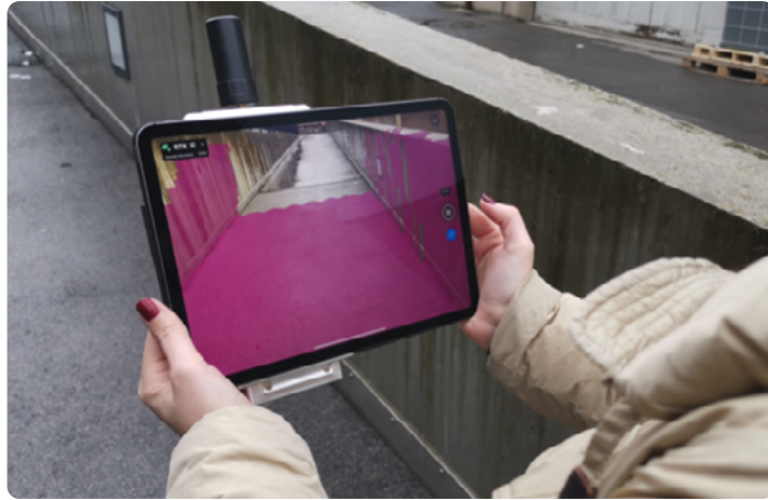
Figure 10: Acquisition of the Pix4D office dataset with the Pix4Dcatch+viDoc®.
